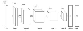
Figure 2: The convolutional neural network after modifying VGG CNN-S
